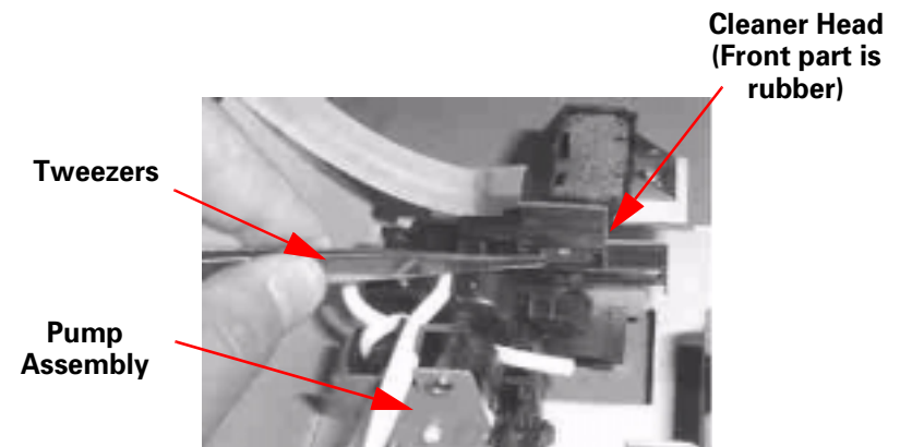
Figure 4-74. Removing the Cleaner Head
