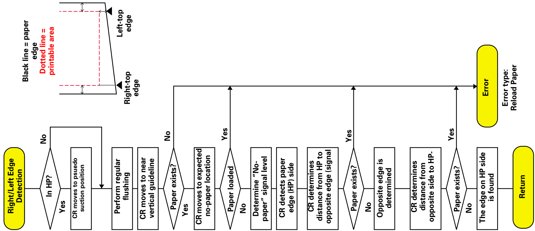
Figure 2-19. Paper Size Detection - R/L edges
