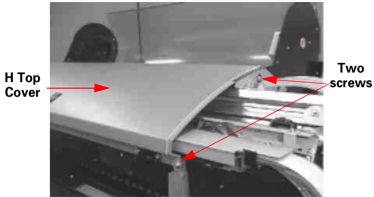
Figure 4-13. H Top Cover Removal on right side
